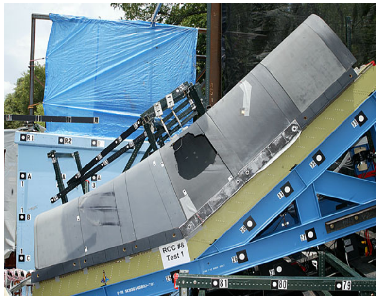
Figure 2: Results from the Foam-Impact Test of the Columbia Debris Strike. Source: NASA Image.
