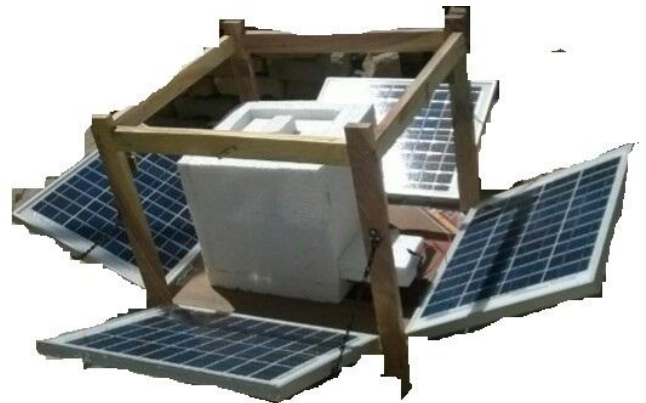
Figure 3: Layout of Solar Powered Icebox
