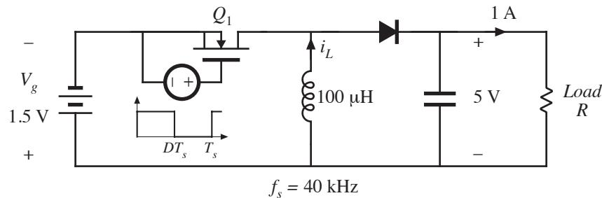
A suitable transistor is found having an on-resistance of 8 milliohms, and a Schottky diode is found that has a forward voltage drop of 0.4 V. The on-resistance of the Schottky diode may be ignored.
