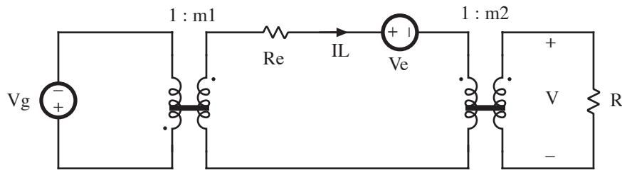
For questions 1 to 4, you are asked to enter mathematical expressions for the elements in this model. The effective turns ratios are functions of only the duty cycle  $D$ , while the effective loss elements  $Re$  and  $Ve$  are functions of the duty cycle  $D$  and the loss elements, but no other quantities.
