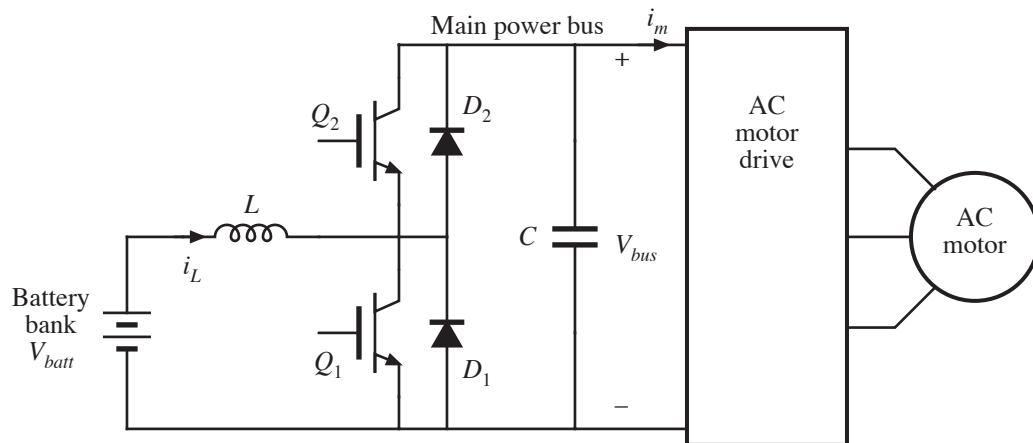
When the vehicle is accelerating, power is drawn out of the battery bank, and the converter boosts the battery voltage  $V_{batt}$  to the dc bus voltage  $V_{bus}$ . The inductor current  $i_L$  is positive under these conditions, and transistor  $Q_1$  conducts during the first interval for  $0 < t < DT_s$ . Diode  $D_2$  conducts during the second interval for  $DT_s < t < T_s$ . Transistor  $Q_2$  and diode  $D_1$  do not conduct for this case.
