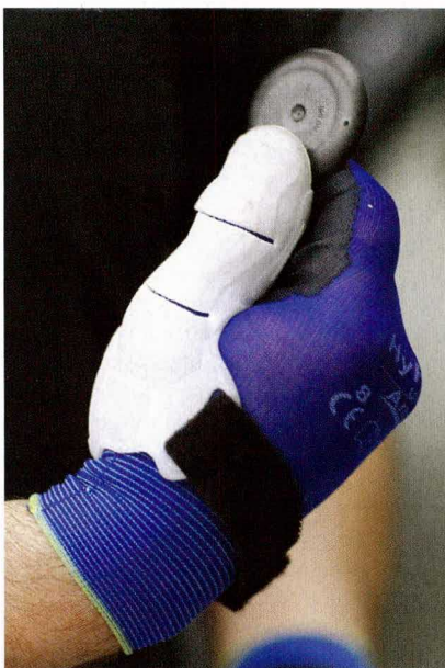
Figure 2. 3D-Printed orthotic finger cot Courtesy of BMW
