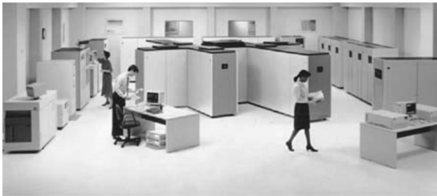
FIGURE 1.3 Inside the Glass House: Series Bipolar Processor Mainframe Computers, Circa 1990–1994 (IBM. Reproduced with permission.)
