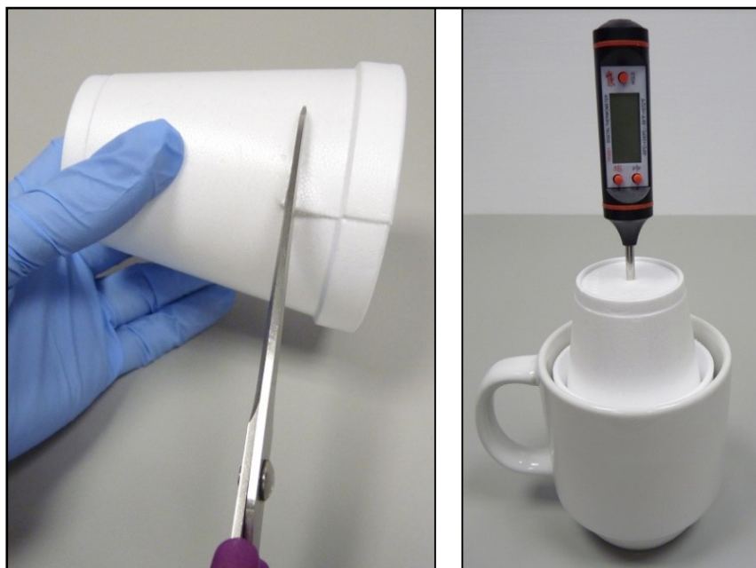
Figure 4. Calorimeter. A. Cutting off 3 cm of the top of a foam cup. B. Complete setup for calorimeter.
