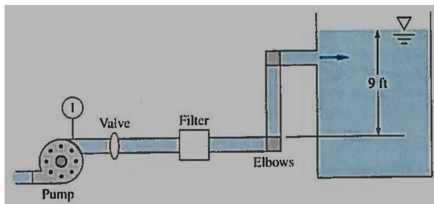
Given: The pipeline sketched is reinforced concrete (2 mm  $\varepsilon$ ), and the pressure head leaving the pump is 75 feet. The system delivers 8 cfs of 20 deg C water to the reservoir. The coordinates of the fittings are:
