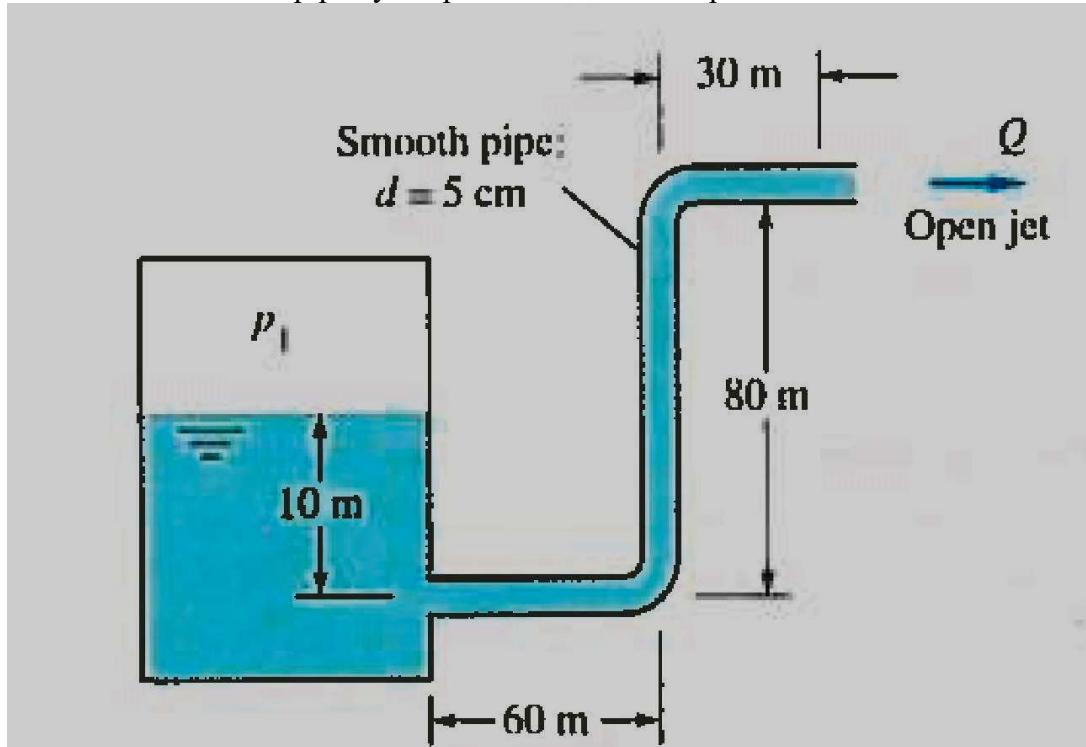
Required: (a) What is the discharge? (b) What is the shear stress 1 cm from the pipe wall? (c) What is the velocity at the edge of the boundary layer?
