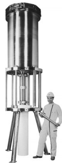
Figure 22-14 A 300-liter preparative chromatography column can purify a kilogram of material. [Courtesy Prochrom, Inc., Indianapolis, IN.]
