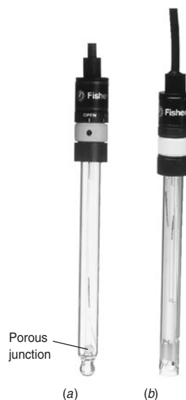
Figure 15-8 (a) Glass-body combination electrode with pH-sensitive glass bulb at the bottom. The porous junction is the salt bridge to the reference electrode compartment. (b) Polymer body surrounds glass electrode to protect the delicate bulb. [Fisher Scientific, Pittsburgh, PA.]
