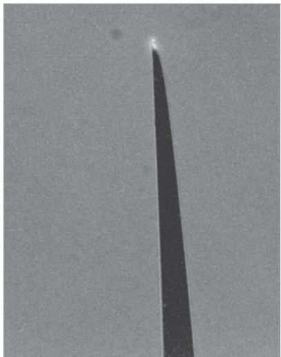
Micrograph shows light emitted from the tip of an optical fiber inserted into a rat embryo. The emission spectrum depends on the pH of fluid surrounding the fiber. Prior to the development of this microscopic method, 1 000 embryos had to be homogenized for a single measurement. [Courtesy R. Kopelman and W. Tan, University of Michigan.]
