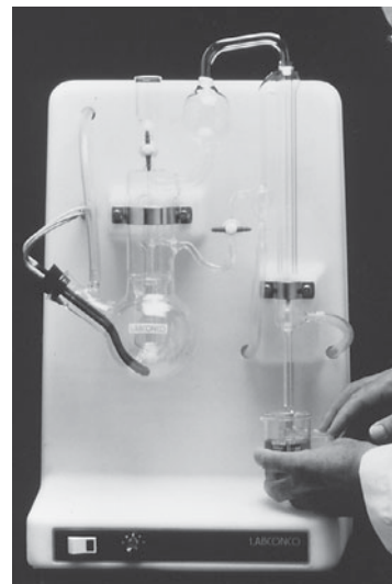
Figure 10-9 Kjeldahl distillation unit employs electric immersion heater in flask at left to carry out distillation in 5 min. Beaker at right collects liberated NH 3 in standard HCl. [Fisher Scientific, Pittsburgh, PA.]
