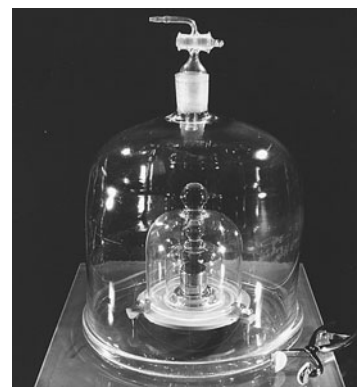
Figure 1-1 Of the fundamental SI units in Table 1-1, only the kilogram is defined by an artifact rather than by a reproducible physical measurement. The international kilogram in France, made from a Pt-Ir alloy in 1885, has been removed from its protective enclosure to be weighed against working copies only in 1890, 1948, and 1992. Its mass could change from reaction with the atmosphere or from wear, so there is research to define a standard for mass based on measurements that should not change over time. [Bureau International des Poids et Mesures.]
