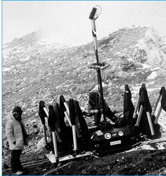
Robot Dante was equipped with a gas chromatograph to sample emissions from volcanic Mt. Erebus in Antarctica. [Philip R. Kyle, New Mexico Tech.]
