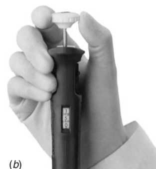
Figure 2-10 (a) Micropipet with disposable plastic tip. (b) Volume selection dial set to 150 \mu\text{L} . [Rainin Instrument Co., Emeryville, CA.]
