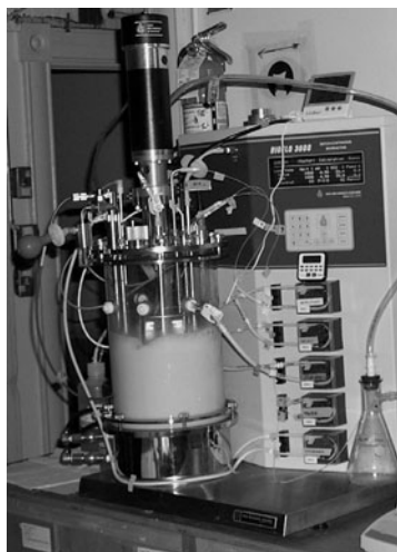
Figure 18-11 Nitrate reductase derived from corn leaves was not easy to produce for \text{NO}_3^- analysis. A stable, recombinant form of the enzyme is made on a commercial scale from yeast cells in the 14-L fermentor in this photo. Recombinant DNA technology permits nitrate reductase genes from Arabidopsis thaliana (a flowering plant also known as thale cress) to be expressed by Pichia pastoris (yeast). [W. H. Campbell, P. Song, and G. G. Barbier, Environ. Chem. Lett. 2006 , 4, 69. Photo courtesy W. H. Campbell, The Nitrate Elimination Co., Lake Linden, MI.]
