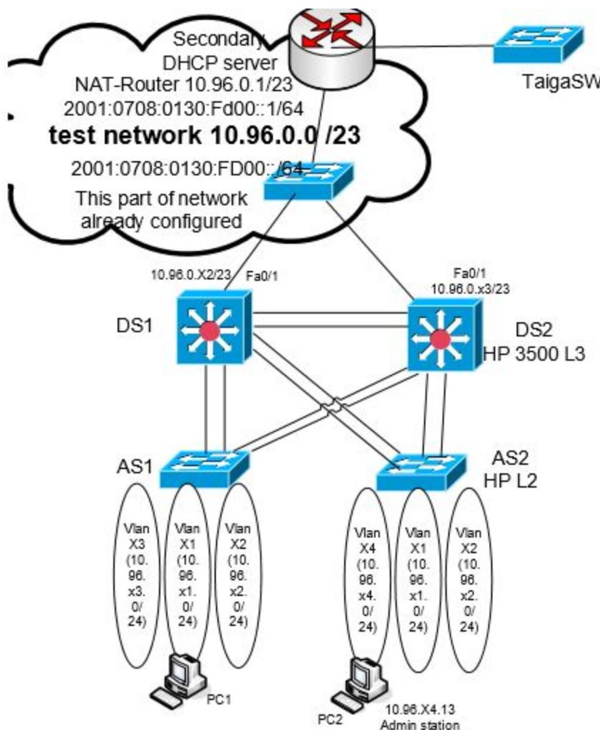
DS1 must be running IOS version 12.2(58) so that it supports VRRP. DS2 switch is HP Procurve 3500 or 3800 series L3 switch. AS2 is HP 2610 or 2620 series L2 switch.
